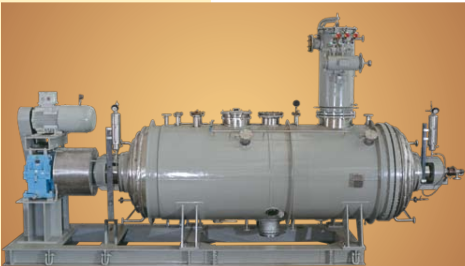
RVD (size 12 m 3 ) manufactured and exported as per PED, CE marked
