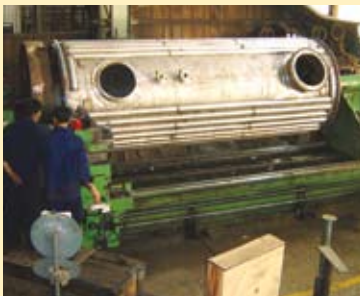
Dryer body being machined
