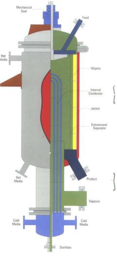
WFE is available in sizes ranging from 0.45  $\text{m}^2$  to 20  $\text{m}^2$  in stainless steel, carbon steel and in other materials such as hastelloy.
